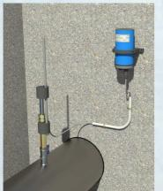
Instrument Data logger GSM/GPRS link box
